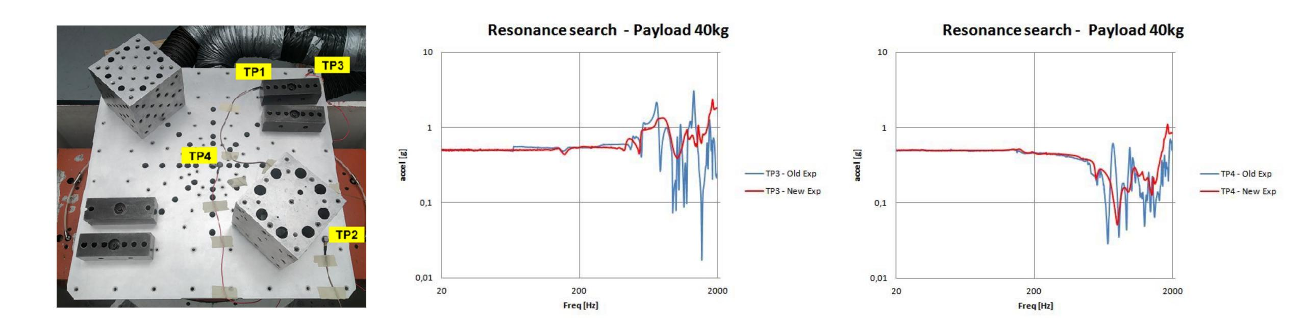
The **Expander Redesign** has been tested at Centrotecnica's testing house showing a better overall performance in loaded condition. Less resonance peaks in high frequency region means an easier control.
