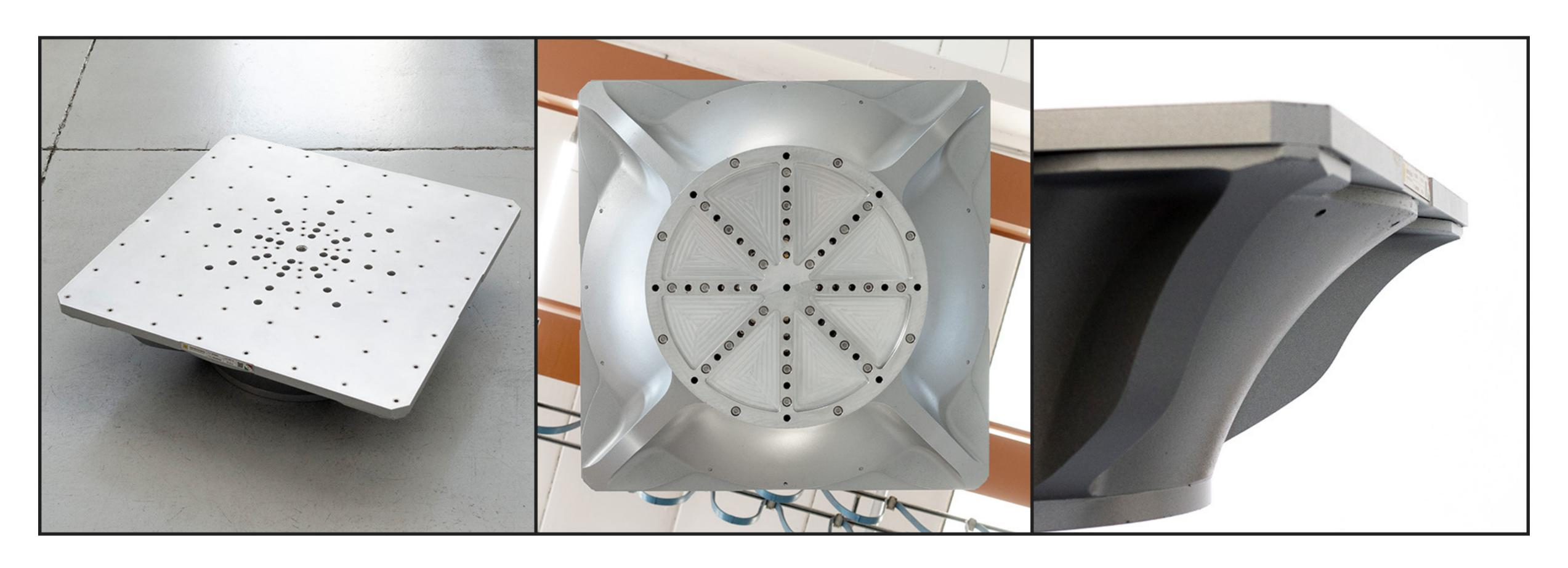
Instant Clamp ready: the solid top plate can be swapped with an Instant Clamp system without adding additional plates. It will make your test faster and cheaper.
